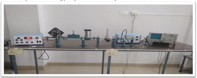
**Facilities:** Klystron Power Supply -2, VSWR Power Supply -2, Tube with mount -2, Directional Coupler-2, Slotted Section -2, Tunable Probe -2, Fixed Attenuator 3dB -2, Fixed Attenuator 6dB -2, Fixed Attenuator 10dB -2, SS Tuner -2, Matched Termination -2, Pin detector -2, Variable matched Terminals -2, Magic Tee -2, Isolators-2port -2, Isolators -3port, Power cords -4, Frequency meters -2, Fan with stand-2, Stands-8, BNC cables -6, Variable attenuator-2.
